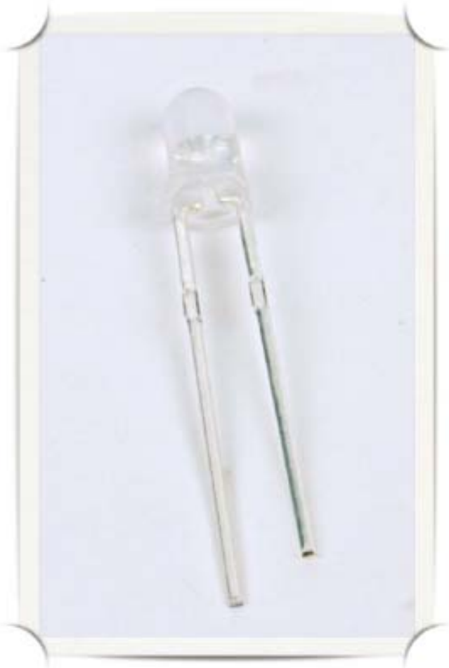
3 mm red-diffused LED. Note the short and long leads: Orientation matters!
