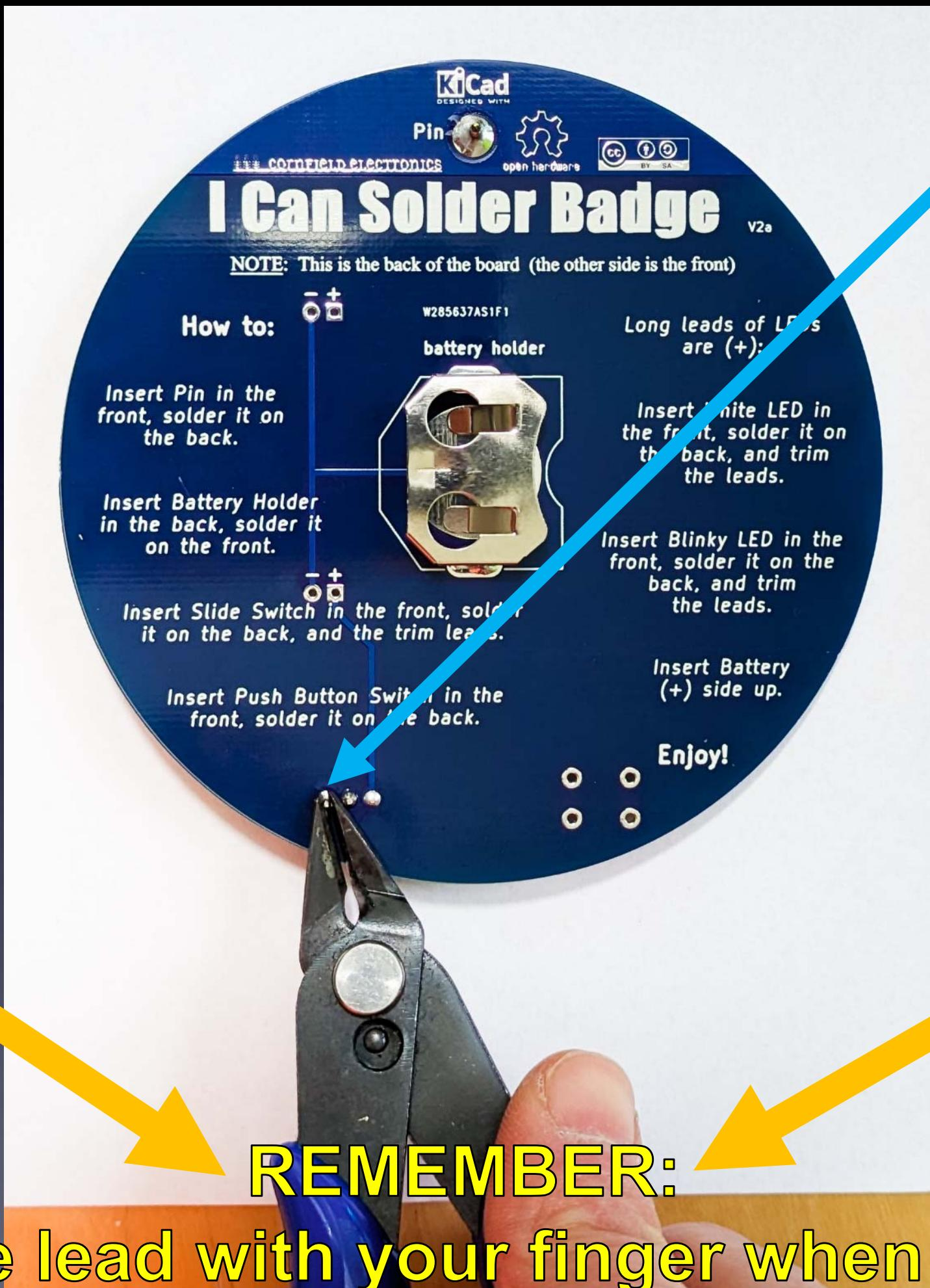
Insert Push Button Switch in the front
