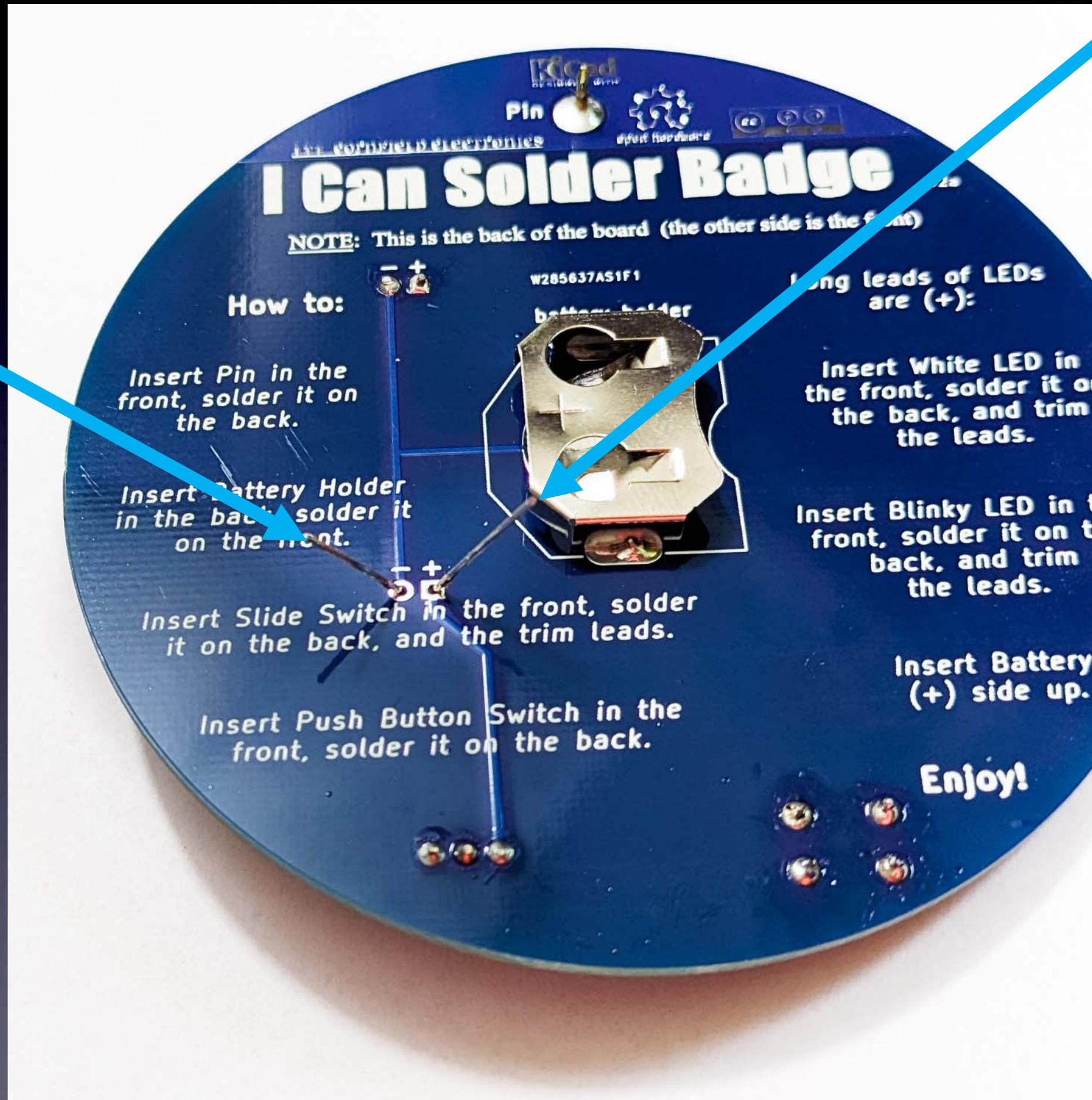
Solder Blinky LED on the back (1<sup>st</sup> pad)
