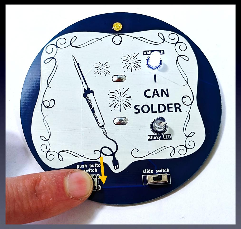
Press Push Button Switch to turn on the White LED
