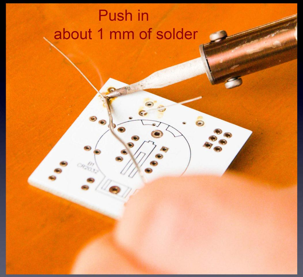
Make sure solder melts on the <u>underside</u> of the soldering iron tip (not the side or top of the soldering iron tip)!
