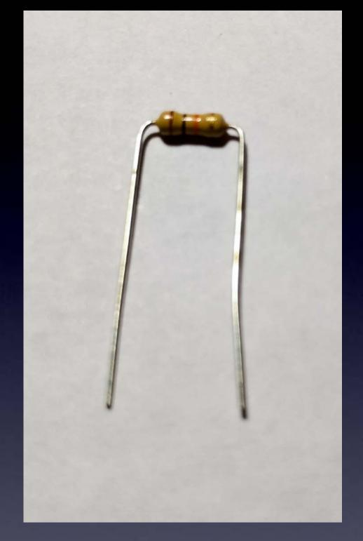
this is how a resistor will look *before* inserting it into the board
