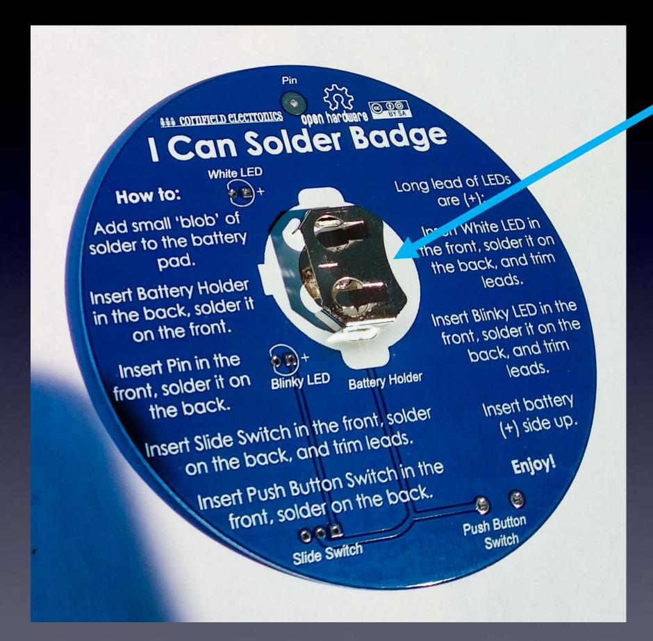
The correct orientation of the battery holder is like this photo
