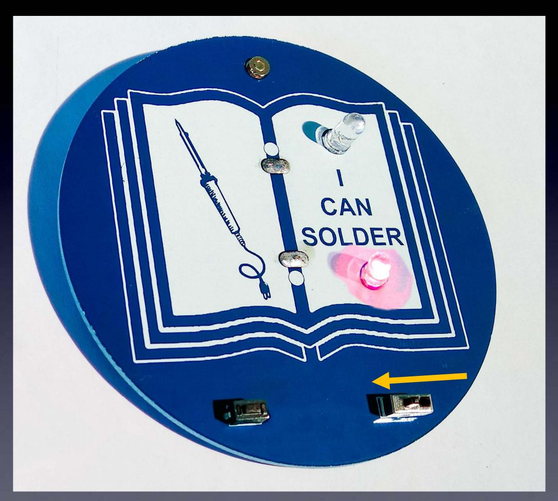
Move Slide Switch to the left to turn on the Blinky LED
