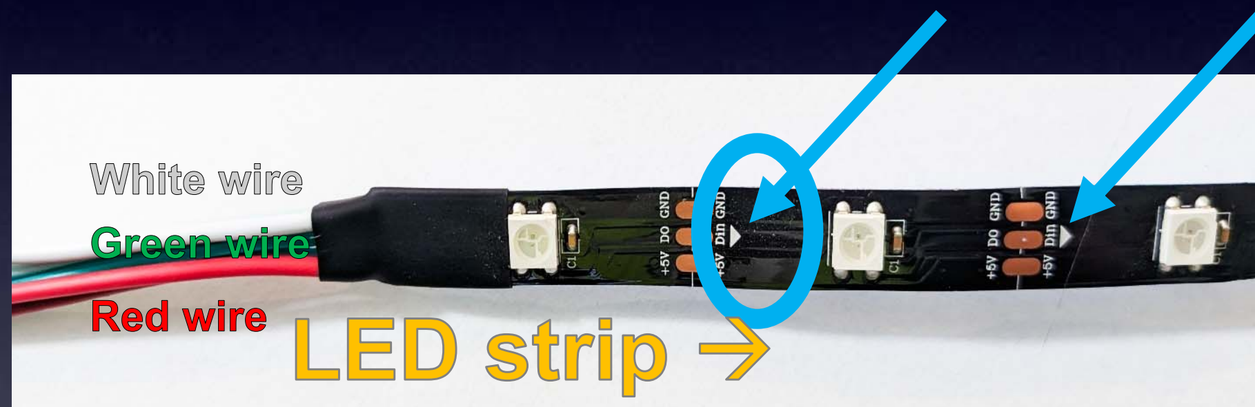
The Input side of the LED Strip
